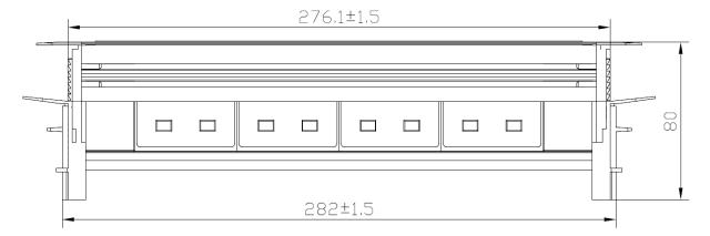
PD Desk units have an integral desk clamp ratchet system, which secures the unit in place. Insert the PD Desk unit into a desk cut-out, then attach the ratchet arms from below. Slide the ratchet arms up to secure.
